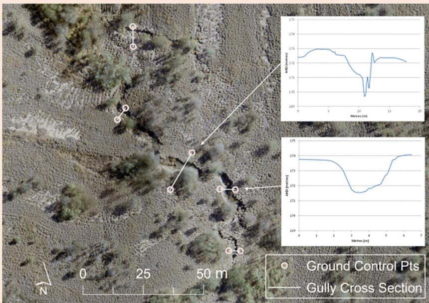
*10 cm UAV orthomosaic showing the presence of an active erosion gully identified through the remote sensing program. This gully is now being monitored over time using UAV orthophoto mosaics, 3D point clouds and field transects to detect long-term change. Graphs on the right show cross-sectional profiles of an active gully, generated using digital surface model measurements at five locations along the length of the gully.*
