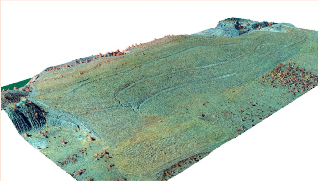
*UAV-generated imagery as a base for 3D false-colour point cloud showing trees, erosion gullies and other features.*
